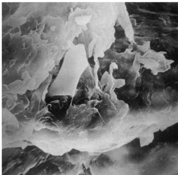
Figure 3 Scanning electron micrograph of 50% untreated perlite-F0753 composite, the impact fractured surface.
