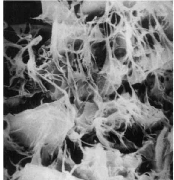
Figure 4 Scanning electron micrograph of 50% hydrolyzed silane treated perlite-F0753 composite, the impact fractured surface.
